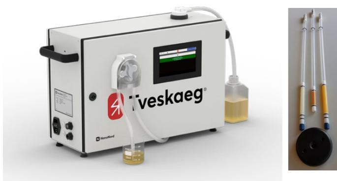
Figure 1. The NanoNord TVESKAEG™ benchtop NMR sensor, based on a 1.5 Tesla magnet and advanced radio-frequency technology, with options for tube (shown in insert to the right) and peristaltic pump (on the front of the spectrometer) sample insertion.
